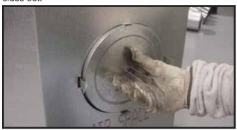
**Figure 7.10** Fold the center parts of the retaining band out and use to remove the vent cap.
